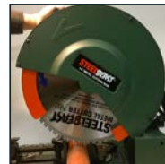
Retracting lower safety guard
