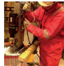
Modified JEI drilling machine and cutter solution for specialist offshore application
